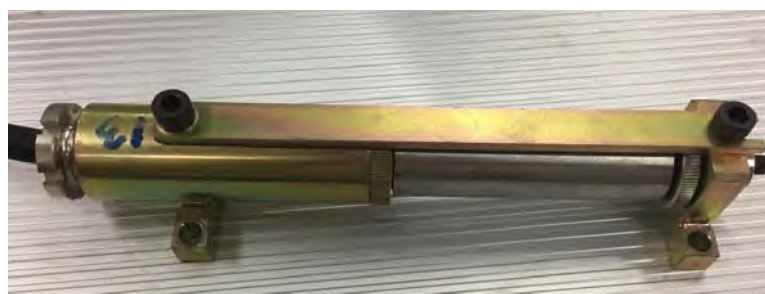
รูปที่ 4.7-3 Surface-mounting type strain Transducer (SSG or SG)
